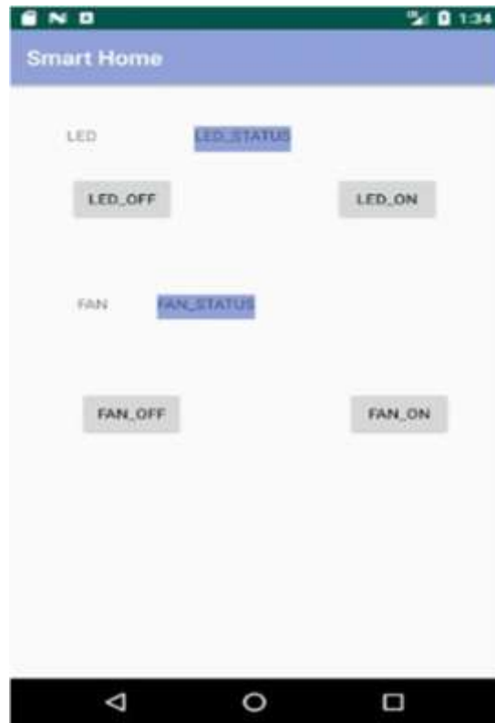
Figure 11 : Home automation system app made with Blynk displaying that the fan is turned on
