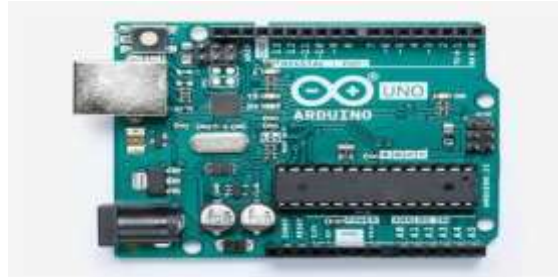
Figure 3: Arduino Atmega 328p
