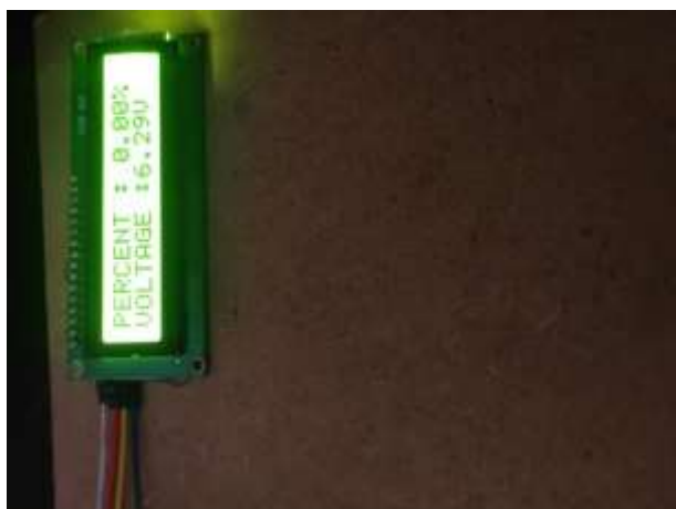
Fig.8 Low battery indication in LCD.
