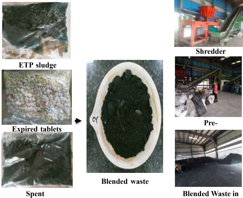
Fig- 1 Pre-Processing of Hazardous Waste at Site
