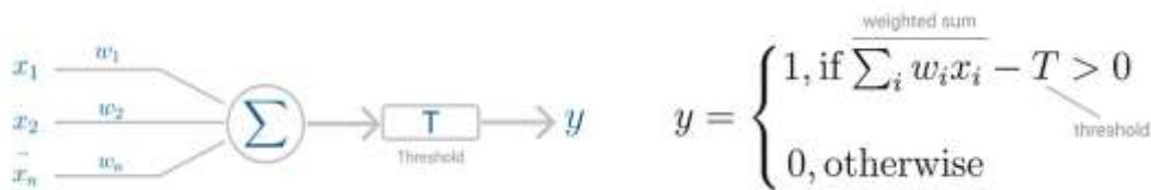
Fig. 3: Perceptron neuron model (left) and threshold logic (right).
