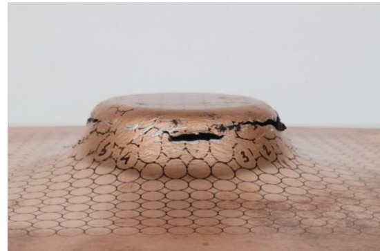
Figure 4: Tearing on Cu-Al arrangement and in Al-Cu arrangement
