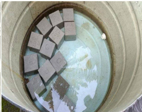
Figure 4: Curing of cubes
