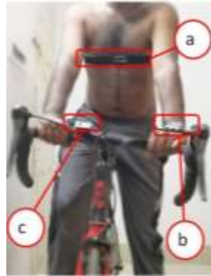
Figure 2. Experiment setup: (a) Polar heart rate sensor unit, (b) Polar training computer (wrist unit), (c) BTwin cycle computer
