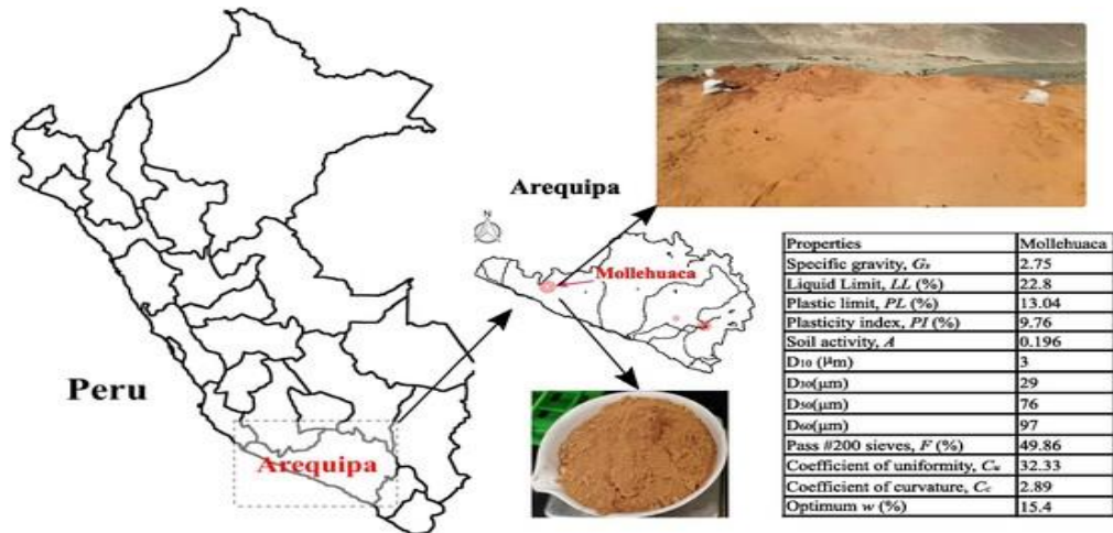
Fig. 1. Diagram of MTs origins and the geotechnical properties
