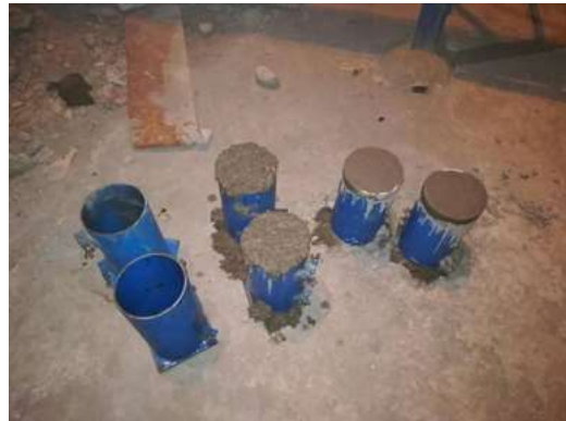
Fig. 11: Casting of cylinder
