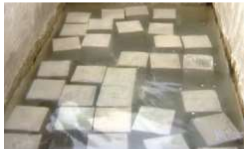
Fig. 12 Specimens in Curing Tank
