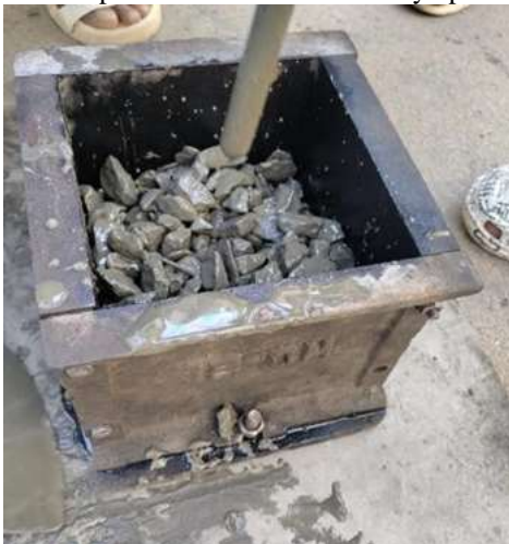
Fig. 10: Casting of cube
