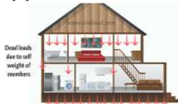
Figure 5: Dead loads on a structure
