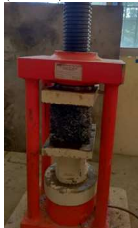
Figure 5: Failure pattern of cube specimen in CTM
