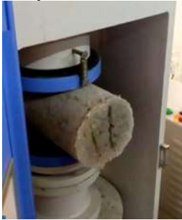
Figure 6: Failure pattern of cylinder specimen in CTM
