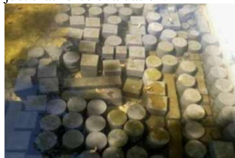
Fig: 8 Curing of concrete moulds
