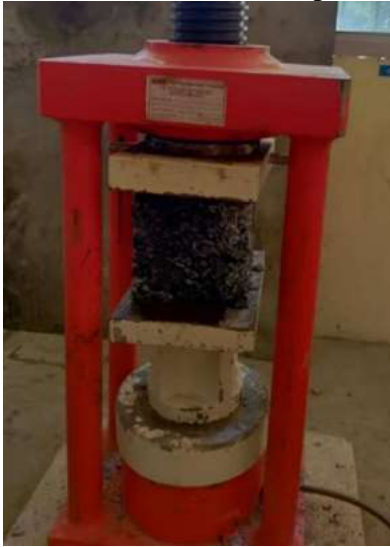
Fig: 9 Compression testing on cubes
