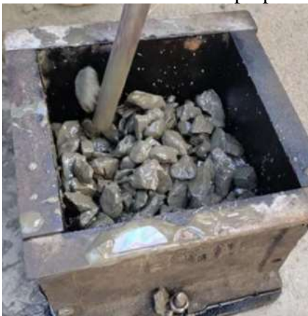
Fig: 6 Moulds for casting (Cubes)
