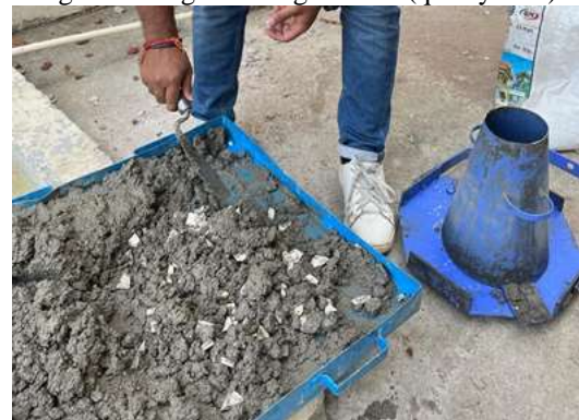
Fig.9: mixing of all ingredients (quarry dust + tile waste)
