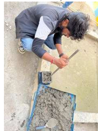
Fig.10: Casting of brick mould
