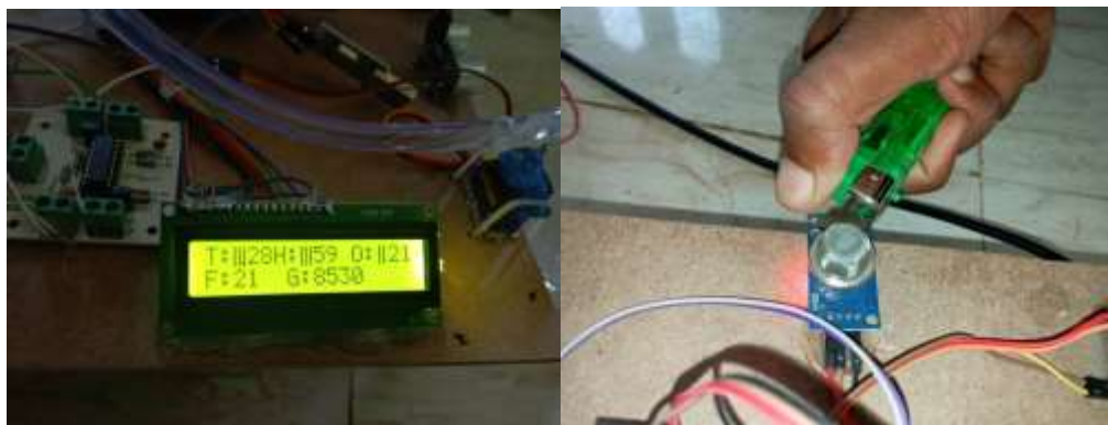
Fig 9. Displaying the Gas values around the robot.
