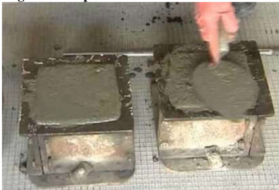
Figure 5. Casting of cubes
