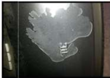
Fig.5 Chipping off (peel off)
