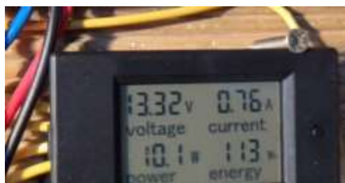
Fig.7. Output of Tulip Wind Driven by PMBLDC generator
