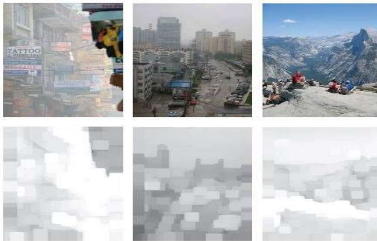
Fig.5. The Light channel of hazy image. From up to down is: (a) Outdoor hazy images. (b) The light channel
