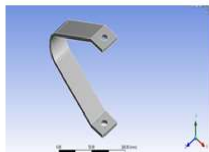
Fig. 2 Geometry of Main Leaf Spring. Fig. 3 Geometry of V- Shape Strip Spring.
