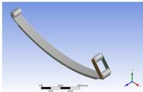
Fig. 2 Geometry of Main Leaf Spring. Fig. 3 Geometry of V- Shape Strip Spring.
