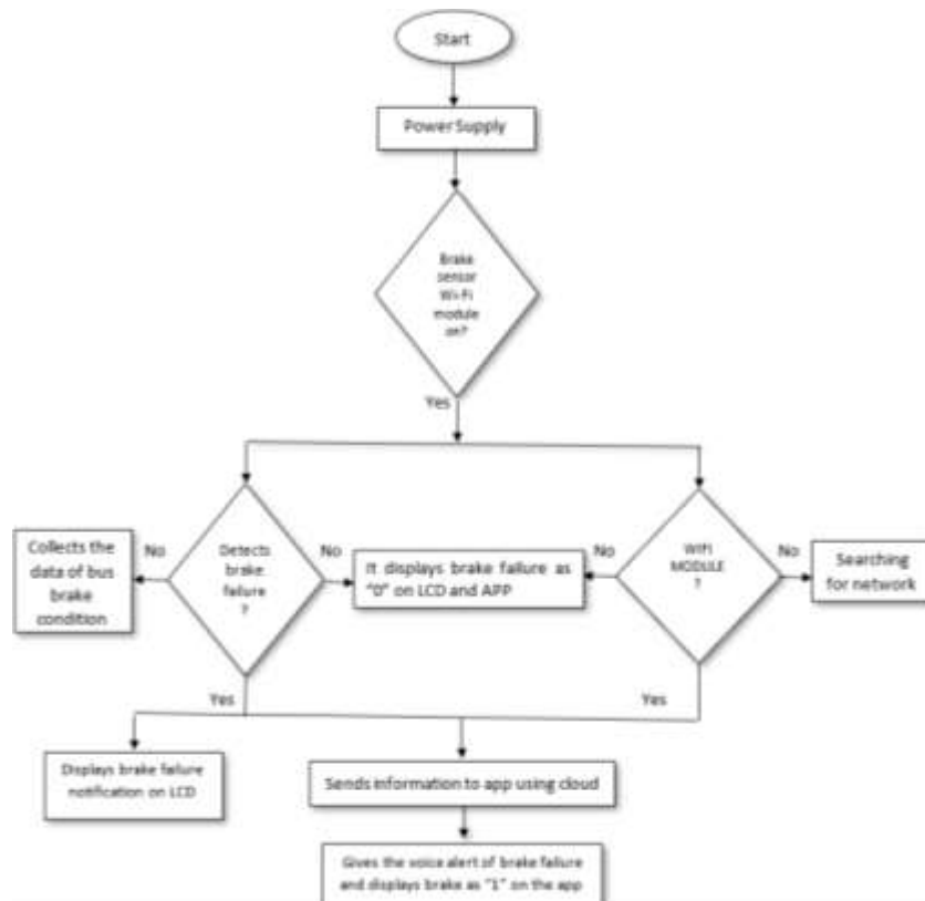
Figure 5: Flow chart of Brake failure detection
