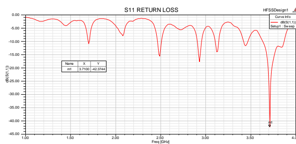
Fig. 4a Return Losses for Circle cut MSPA Array
