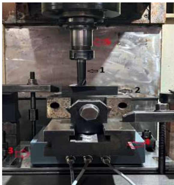
(1) Solid Carbide End mill , (2) CFRP Material, (3) MillingTool Dynamometer , (4) Precision Modular Vice, (5) BT40 Collet Chuck Holder
