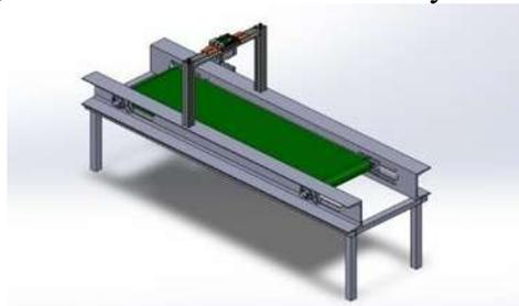
Figure 2: 3D design of the conveyor system.
