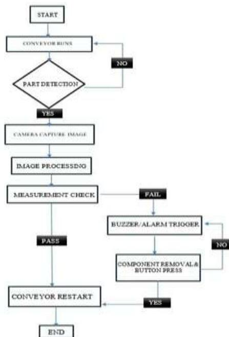
Figure 3: Software processing workflow.
