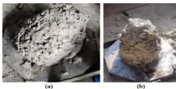
Figure 5 Slump test of (a) GPC with FA and (b) GPC with FA 1 GGBS
