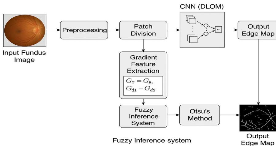
Fig. 1. Block diagram of the DGOFED pipeline.
