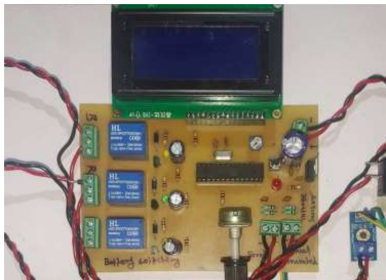
Fig. 6: Embedded Test bed on PCB Design
