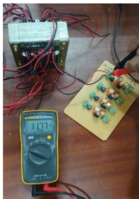
Fig 4: Input voltage of rectifier
