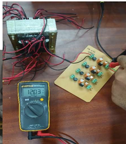
Fig.6 Output voltage of rectifier
