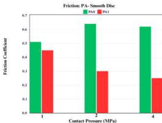
Fig 6: Friction coefficient of PA composite against smooth steel disc
