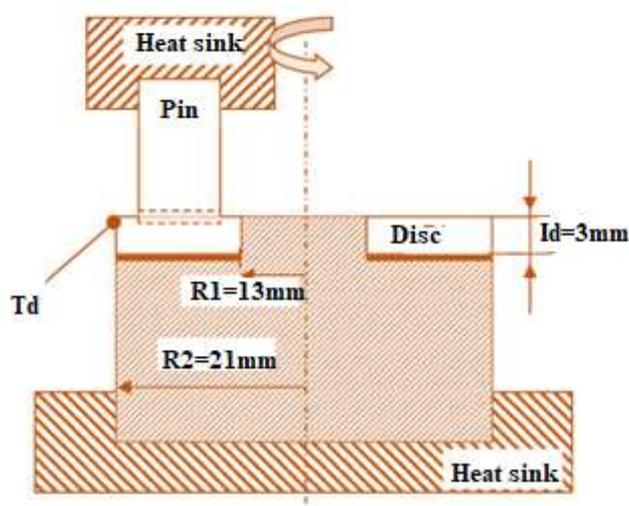
Fig 2: The sliding wear set-up for cross-sectional schematic model
