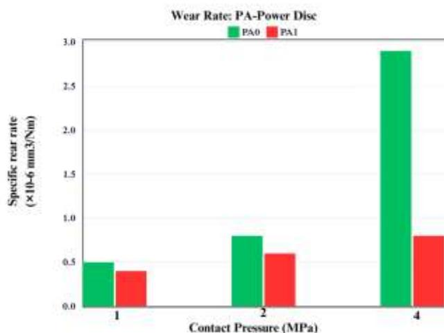
Fig 3: The sliding wear test results are shown as the average of two tests, with the error bars indicating the respective standard deviations. The PA composites' wear rates versus certain materials of rough steel disc
