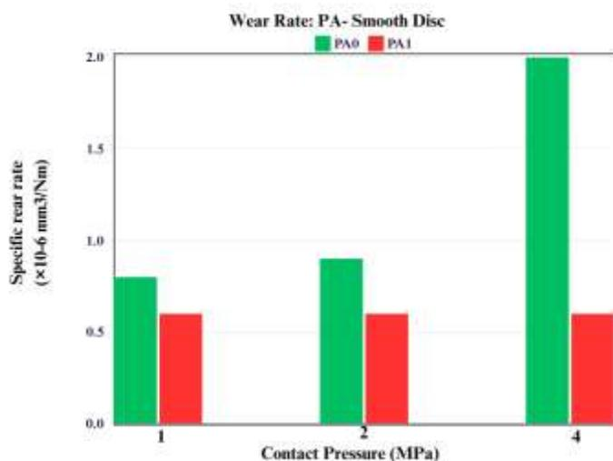
Fig 4: The sliding wear test results are shown as the average of two tests, with the error bars indicating the respective standard deviations. The PA composites' wear rates versus certain materials of smooth steel disc
