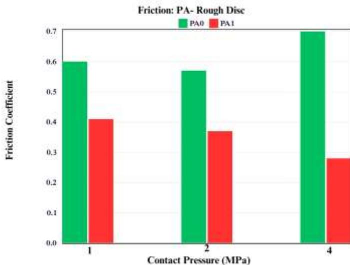
Fig 5: Friction coefficient of PA composite against rough steel disc
