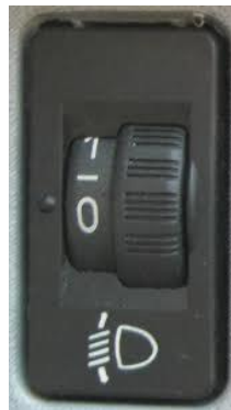
Fig. 2. Manual headlamp levelling switch placed near the driver
