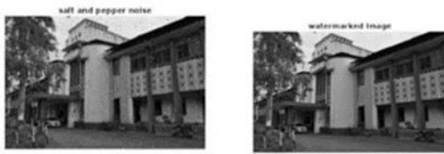
Image with noise watermarked image Attack level-0.01db, Accuracy-98.01%, PSNR-49.7432 and BER-0.52822, fig 4.1.2(a)
