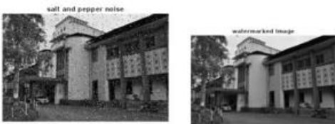
Image with noise watermarked image Attack level-0.04db, Accuracy-95.98%, PSNR-49.7432 and BER-0.53653,fig 4.1.2(d)
