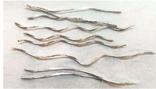
Figure 12: Long continuous chips
