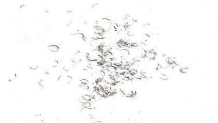
Figure 13: Asymmetrical continuous chips Figure 14: Discontinuous chips
