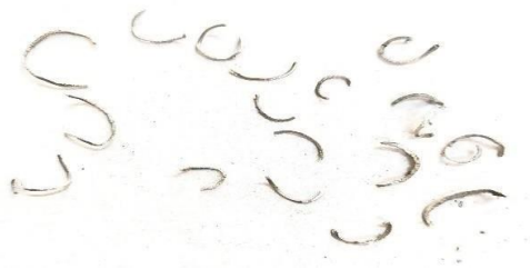
Figure 13: Asymmetrical continuous chips Figure 14: Discontinuous chips
