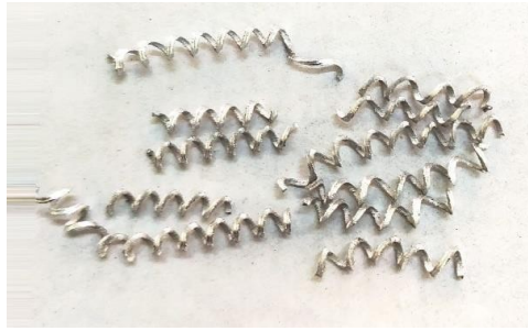
Figure 11: Spiral continuous chips
