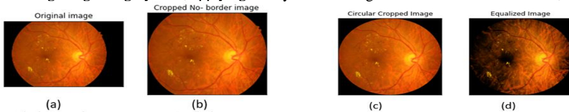
Figure.3: IDRID database results. (a) Original image. (b) No-border image. (c) Circular crop image. (d) Histogram equalization
