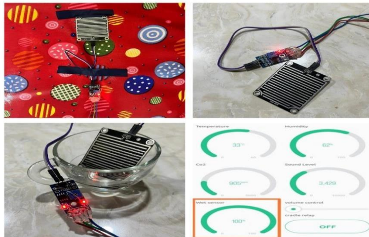
Fig8: Detection of Moisture and output in Blynk app
