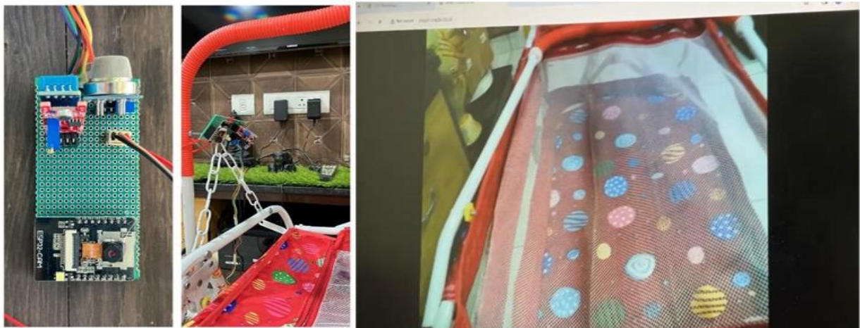
Fig6:ESP32 Cam Setup and Remote Monitoring of Baby's Cradle through Camera
