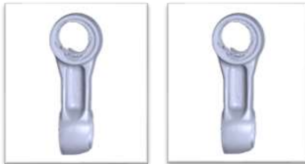
Figure 1 Model of damaged high-speed coupling arm
