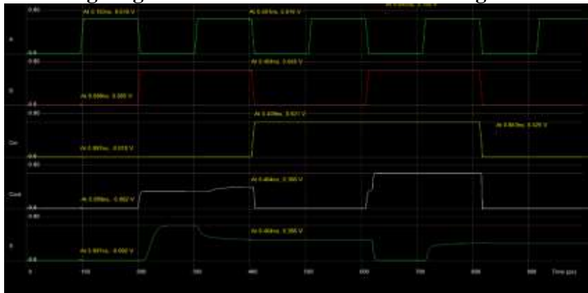
Figure 3(b): Backend layout timing diagram of 10 transistor full adder using 7-nm technology
