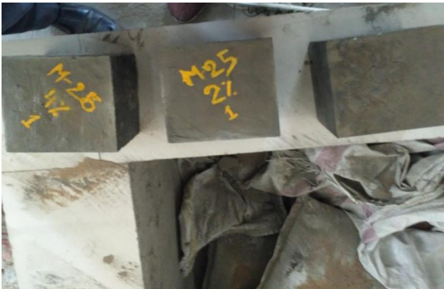
Figure 3: Cubes with Partially Replaced PVC
