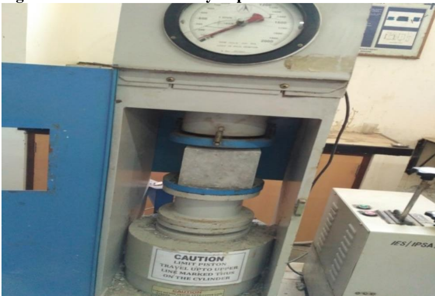
Figure 4: Cube testing on CTM
