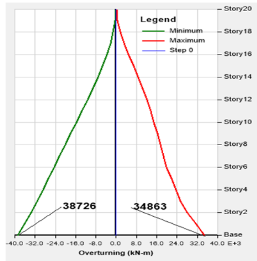
Figure 12. Overturning Moment for Conventional Building
