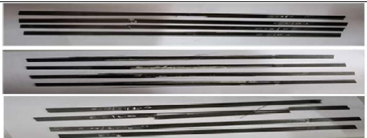
Fig.6. Failure specimens of hybrid composites
