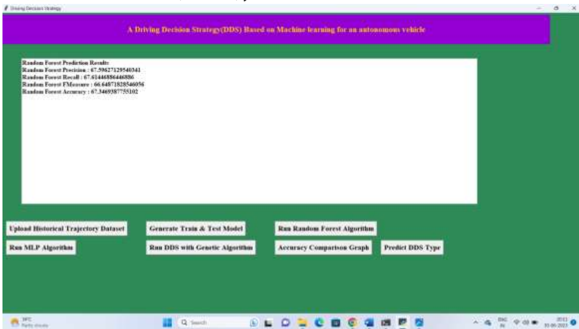
Fig 4.3 In above screen we calculated random forest accuracy, precision, recall and fmeasure and random forest got 67% prediction accuracy. Now click on ‘Run MLP Algorithm’ button to train MLP model and to calculate its accuracy
