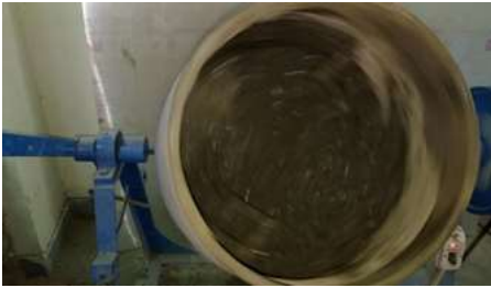
FIG NO: 3: CONCRETE MIXER
