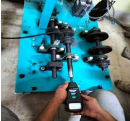
Fig.1.3: Finding speed with the help of Tachometer
