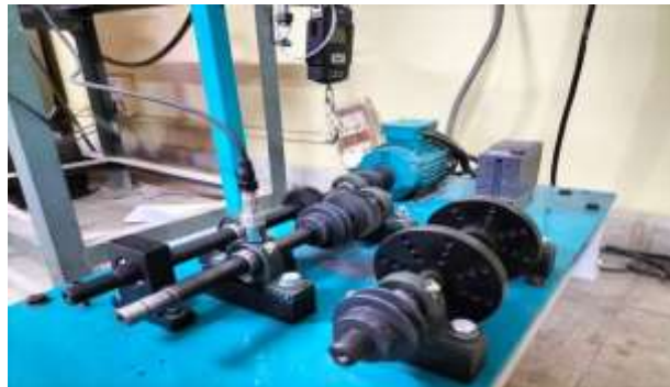
Fig.1.1: Experimental Setup with accelerometer mounted on it
