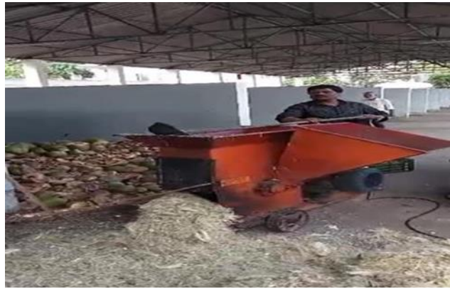
Figure3.14 Processed through Shredder Machine
