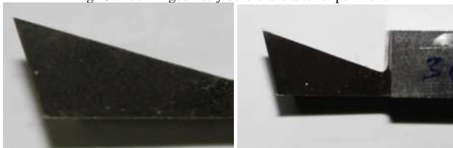
Fig 13: Tool 11 geometry before and after experiment
