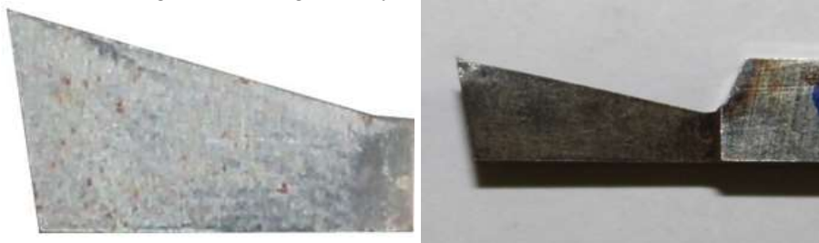
Fig 26: Tool 8 geometry before and after experiment
