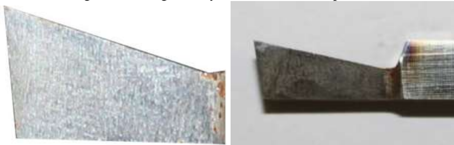
Fig 25: Tool 7 geometry before and after experiment
