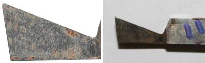
Fig 29: Tool 11 geometry before and after experiment
