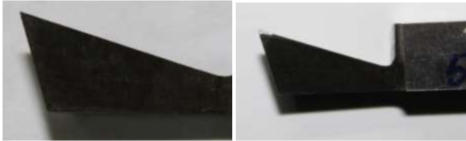
Fig 16: Tool 14 geometry before and after experiment
