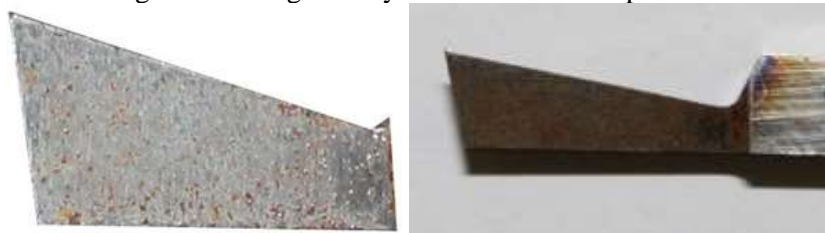
Fig 27: Tool 9 geometry before and after experiment
