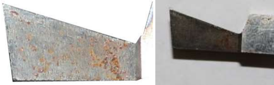
Fig 20: Tool 2 geometry before and after experiment
