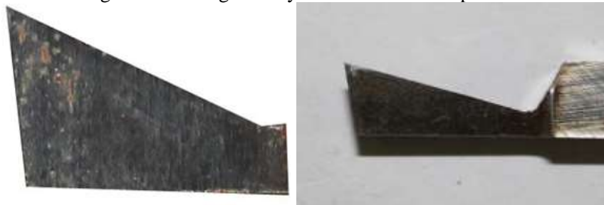
Fig 33: Tool 15 geometry before and after experiment
