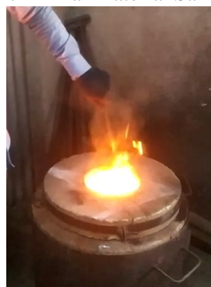
Fig. 19 – Addition of Reinforcements
