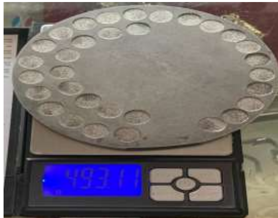
Figure 6. Experimentation on Superni90 work material with Aluminum7178 using EDM
