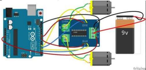
This image shows a wiring diagram for connecting an Arduino Uno to a motor driver (HC05) and two DC motors, powered by a 9V CHARGABLE battery. Here's a breakdown of the connections:
