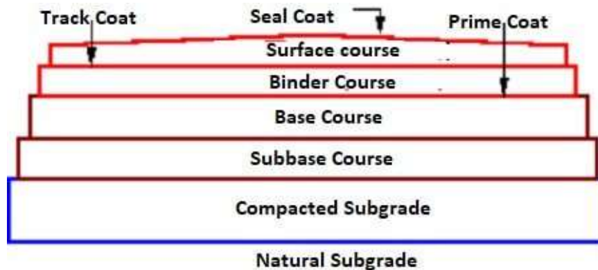
Fig 0.1: Typical layers of flexible pavement
