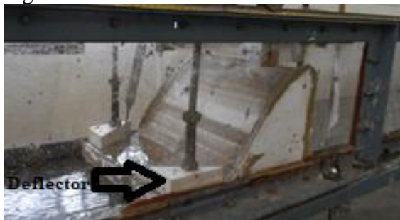
Figure 8: Side view of DSB model installed in flume.
