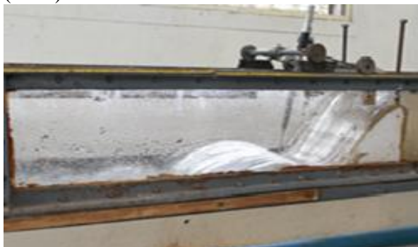
Figure 7: Side view of CSB model installed in flume.
