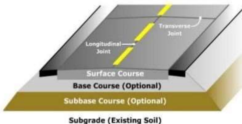
Figure 2- Rigid Pavement Typical Cross-section
