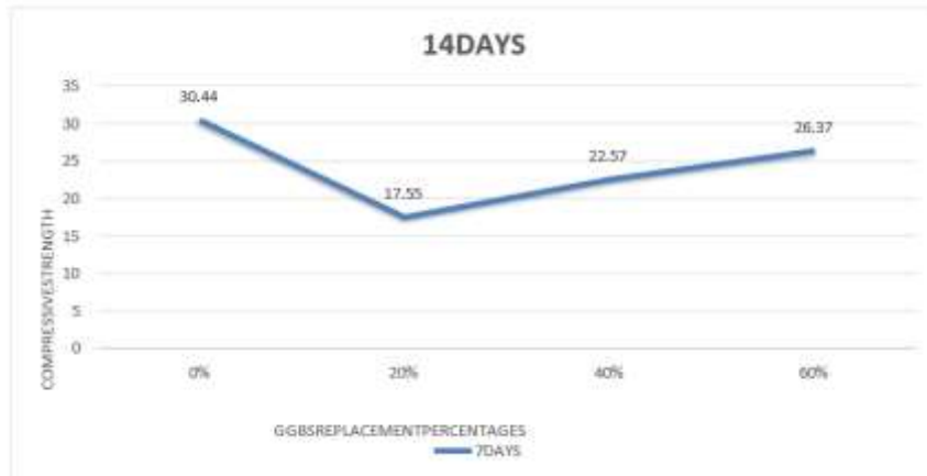
Fig 9. A graph representation of 14 days compressive strength test results
