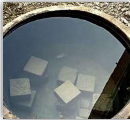
Fig 6. Curing of cubes
